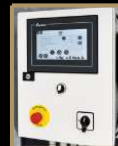
Programmable computer for the horsewalker. It allows you to set the walk and trot frequencies and turnaround times. It is suitable for making personalised programs for your horses
